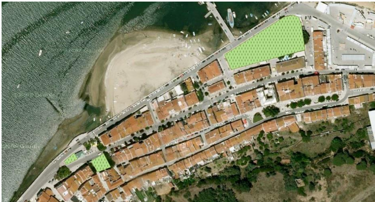
Figure 5.10 – Detention basin technique applied in QGIS
