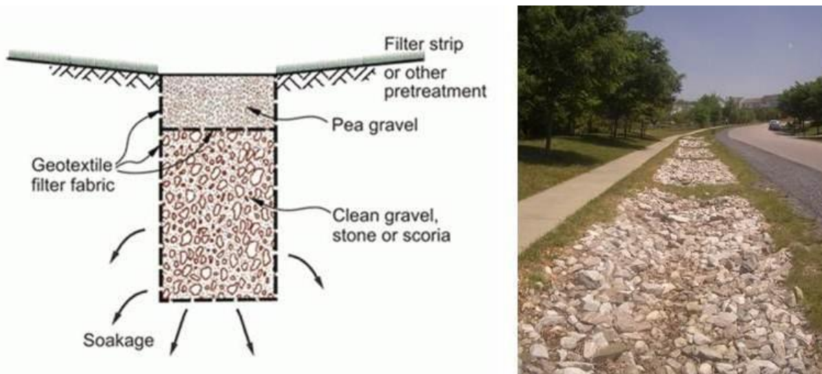
Figure 2.22 - Infiltration trench ( www.sswm.info/ , 2015)
