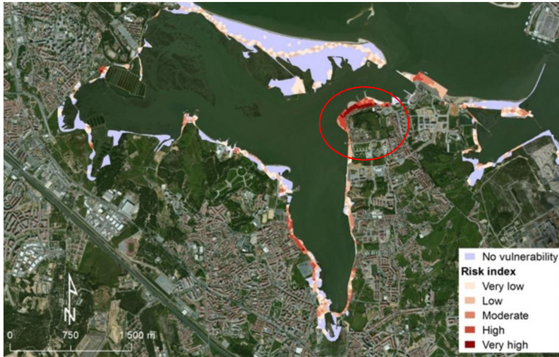
Figure 4.5 - Risk index in the Seixal municipality for a 100-year return period scenario (Project Molines)
